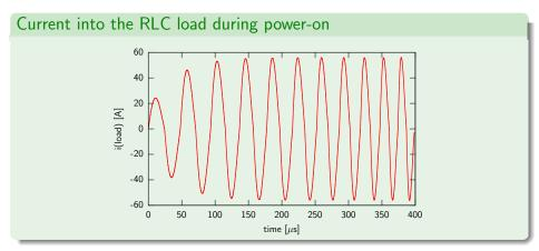
A sweep of the inductance of the load has been imposed changing continuosly the oscillating frequency.
