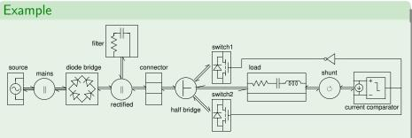
SystemC-WMS modules and wavechannels interconnection diagram
