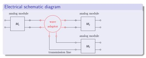
A wavechannel can be represented by a junction box connected to ports by transmission lines
