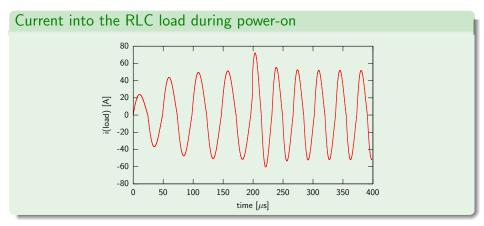
After a 200  $\mu$ s, an abruput change from 80  $\mu$ H to 40  $\mu$ H of the inductance of the load has been imposed.
