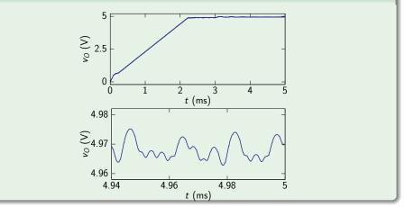
The load voltage during power-on and the load voltage in steady-state,
