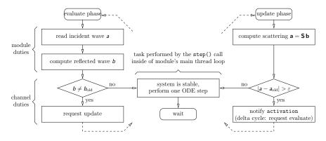
Figure: Sketch of the execution flow inside modules and wavechannels.
