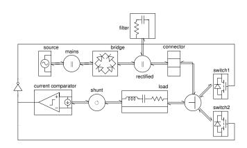
Fig. 3. Self-oscillating half-bridge inverter: SystemC modules and wavechannels interconnection diagram.
