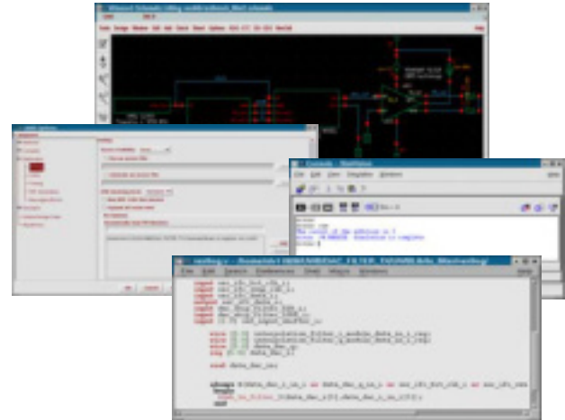
Fig 1. Co-simulation using the Verilog Procedural Interface (VPI)
