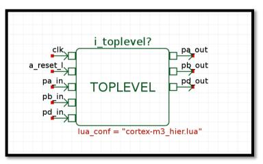
• System configuration via LUA file provide through toplevel parameter
