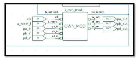
Corresponding Wrapper of the whole Cortex M3 processor exposing the interface Signals
