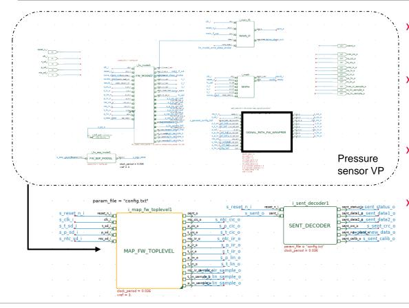
Simple test bench instantiating VP and SENT decoder fulfilling 'checkers' role Stimuli driven programmatically in multiple stimuli files based on application (signal ramp, mid range, signal step etc.) Selection of stimuli done in regression based on implemented test case Rest of VP configuration done through *config.txt* file coupled to model parameters as well as configuration signals in dedicated module
